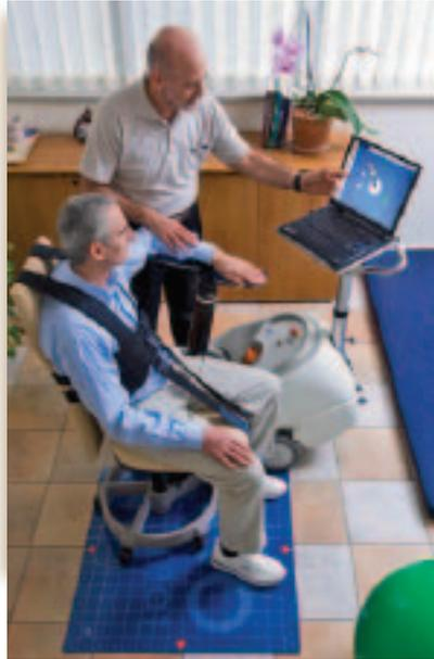
in the motor-driven joints indicate the amount of effort generated by the patient. The device lessens the manual labor needed for therapy,
